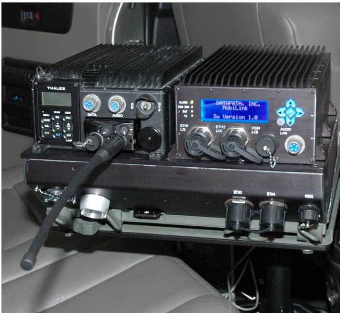
With a low profile, roof-mounted antenna, the DataPath mSAT-XLT mounts in a SINCGARS MT-6352 tray for a compact configuration.
