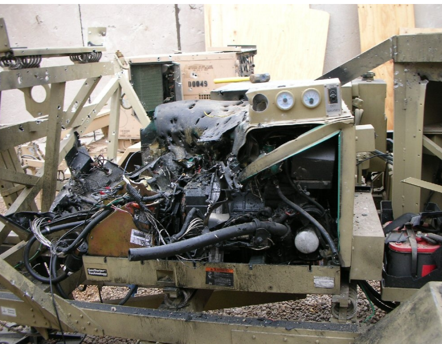
The STT that was severely damaged as the result of a mortar attack.
