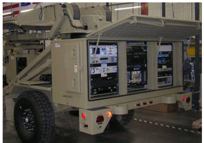
QUALCOMM Deployable Base Station (QDBS) integrated into the middle bay of STT #623 at DataPath's integration and production facility in Duluth, Ga.
